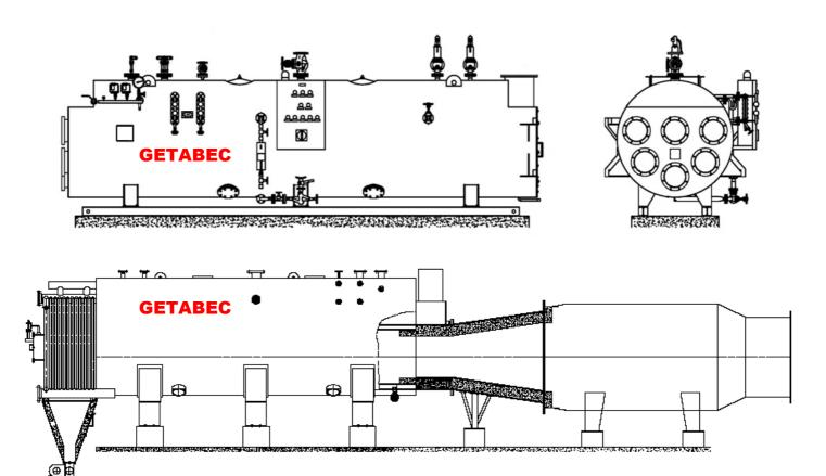
The Waste Heat Recovery Boiler - HRSG from **Getabec** is designed according to the principle of the flame tube/smoke tube boiler. Here, the hot flue gas is directed through pipe bundles, where its heat is transferred to the water inside the boiler body.
